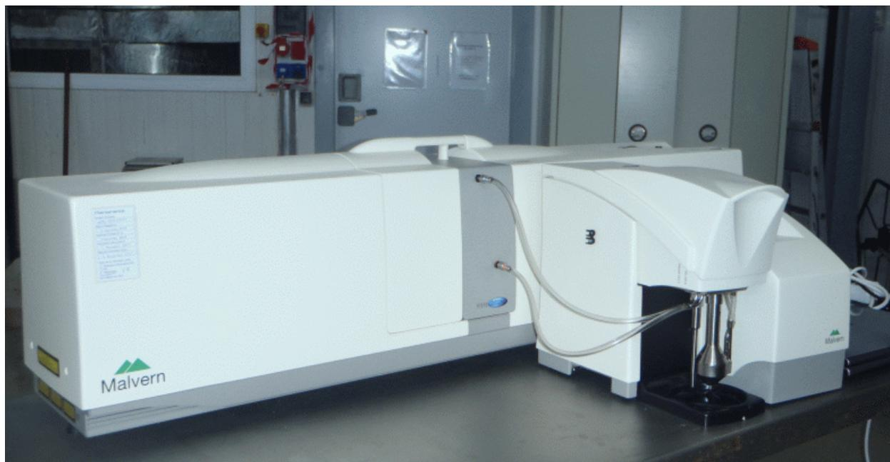
**Figure 4** Laser particle size analyser (optical unit and input system)
